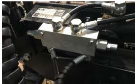
Check valve. Protects your controls.
