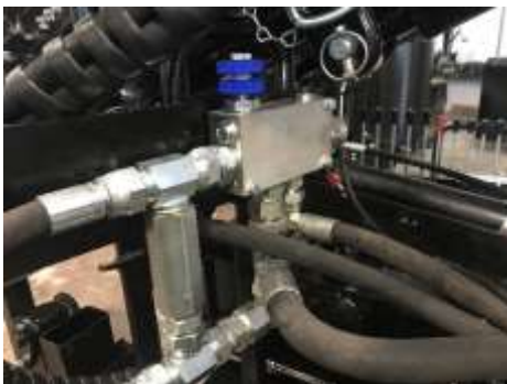
Relief valve (will protect your machine from excessive skid-steer flow). Adjustable.
