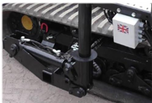
The **wire unroller** is stored on the middle post tray, just insert it into its final position on the side of the machine, at track level. A pin is provided to secure the wire unroller in position. The wire support plate (round plate) provided slides into the long tube. Again, should be no problem.
