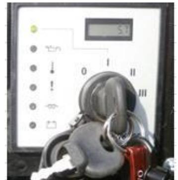
You can adjust the RPM of the engine with the **electric throttle** in the control box (black button as per the picture below)
